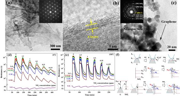
**RESULTS:** (a, b) HR-TEM images of graphene (G), (c) BF-TEM images of 0.5 wt%G/SnO<sub>2</sub>, change in resistance under exposure to NO<sub>2</sub> (0.125 to 5 ppm) of G, SnO<sub>2</sub>, 0.1-5 wt%G/SnO<sub>2</sub> sensors at (d) room temperature (25°C) and (e) the optimal working temperature (150°C), and (f) the energy band models for NO<sub>2</sub> sensing mechanisms of multilayer G, SnO<sub>2</sub> surface, G-SnO<sub>2</sub> interface.
